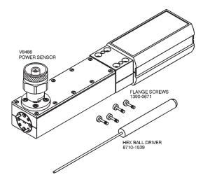
**Dimensions:** width 38 mm (1.5 in"), length 199 mm (7.8 in"), height 60 mm (2.4 in")
